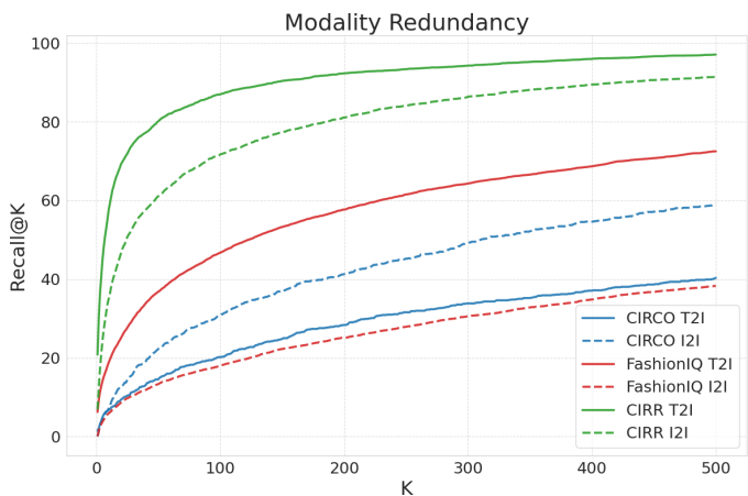
Fig. 7. Evaluation of the modality redundancy of CIRCO, CIRR, and FashionIQ validation sets. Lower values are better. T2I and I2I represent Text-to-Image and Image-to-Text retrieval, respectively.
